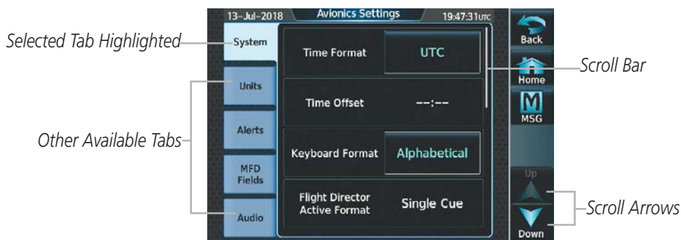
Figure 1-7 Touchscreen Controller with Tabs and Scroll Arrows
