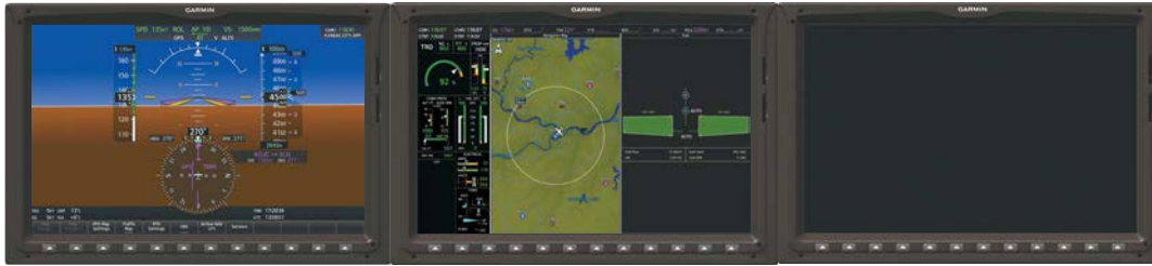
Figure 1-22 Reversionary Mode - PFD2 Failure
