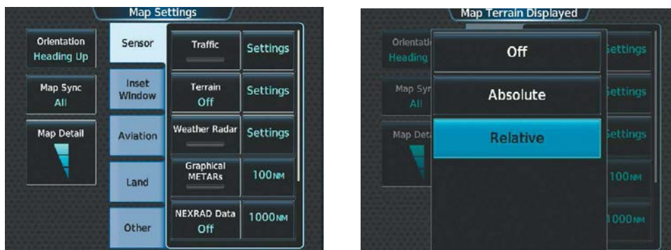
Figure 6-95 Enabling Relative Terrain for the Profile View Inset Window and Navigation Map Pane
