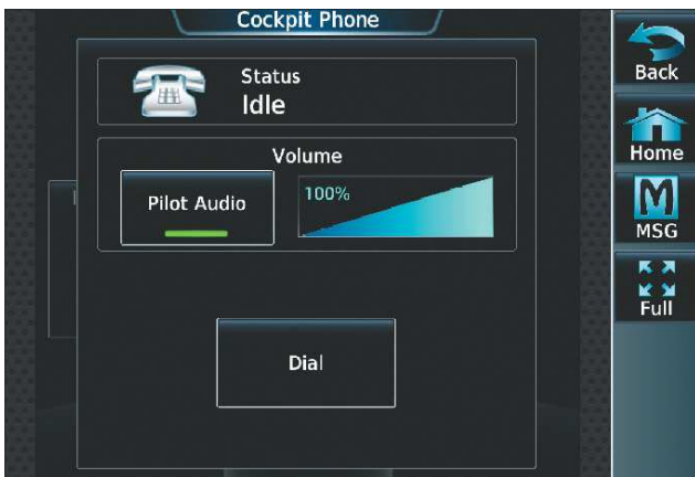
Figure 8-60 Cockpit Telephone Status
