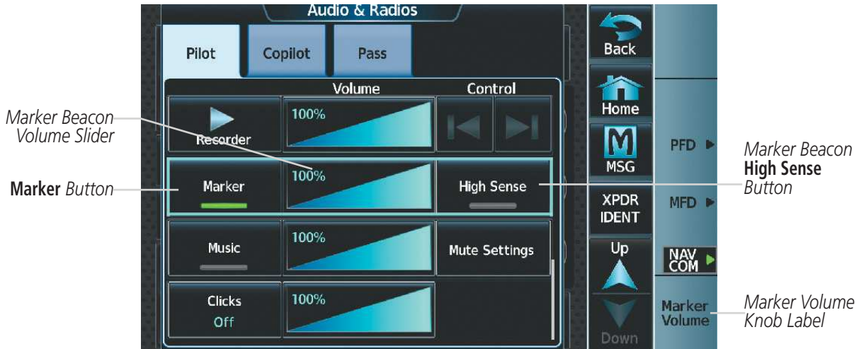
Figure 4-29 Marker Beacon Controls
