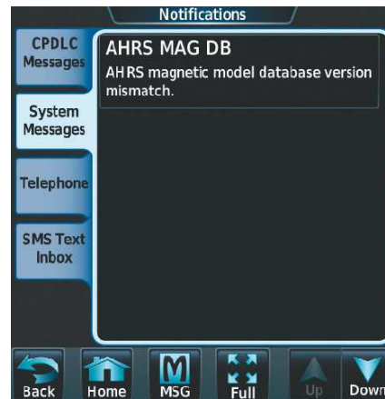
Figure B-18 Database Mismatch Message is Annunciated Before Second GRS is Updated
