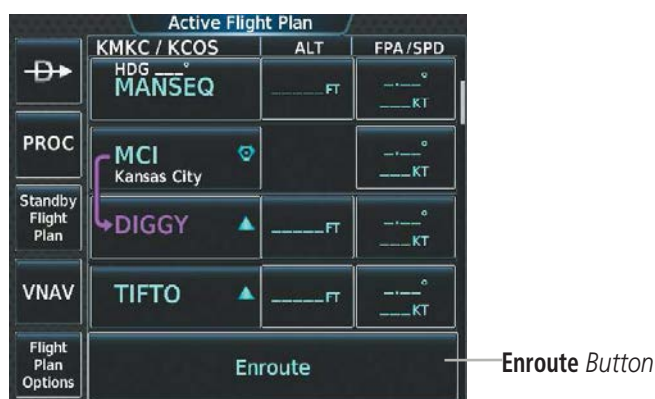
Figure 5-73 'Active Flight Plan' Screen - Adding a Waypoint to the beginning of the Enroute segment of the Flight Plan
