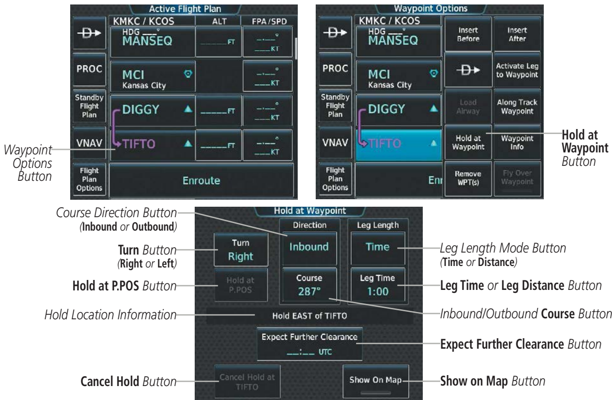
Figure 5-101 Creating a User Defined Holding Pattern at an Active Flight Plan Waypoint
