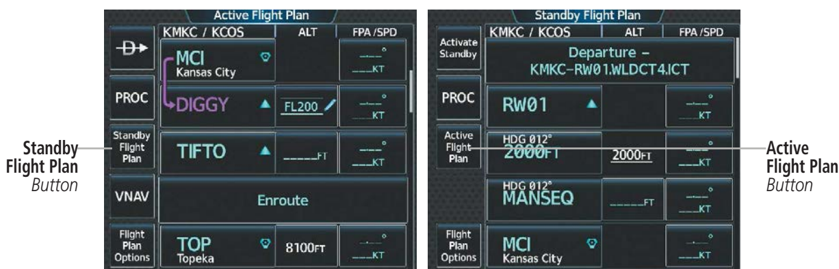
Figure 5-89 Switching between Active and Standby Flight Plan Screen
