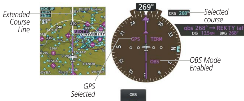
Figure 2-33 Omni-bearing Selector (OBS) Mode Enabled
