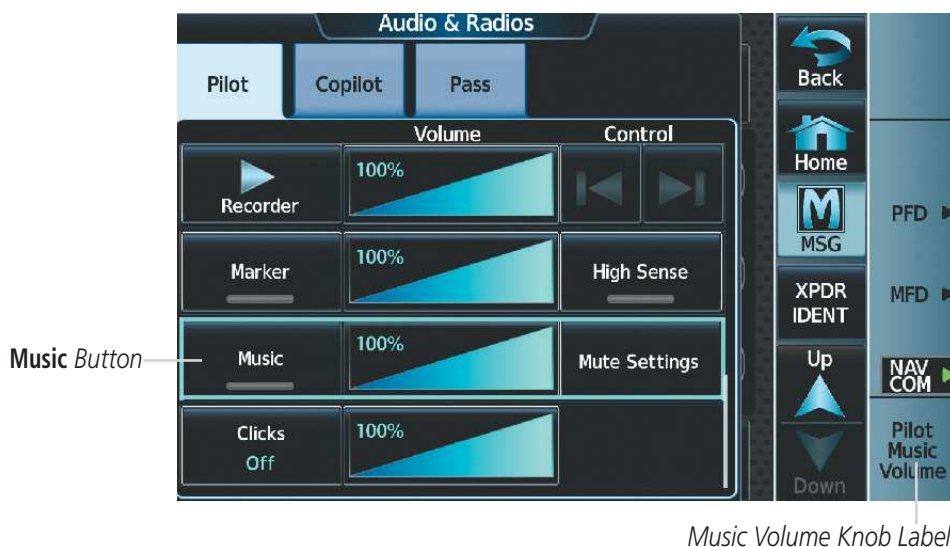
Figure 4-53 Auxiliary Audio Controls
