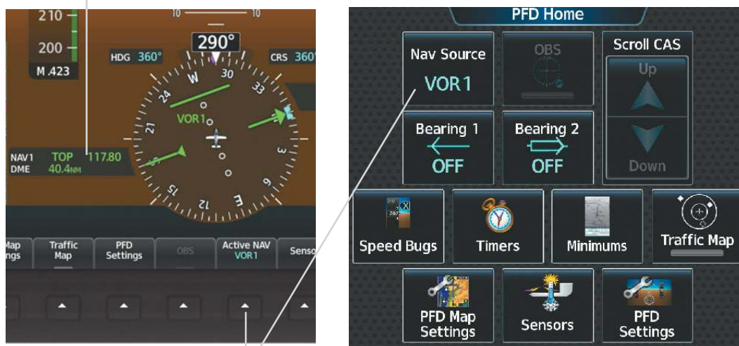
The NAV Radio is selected by touching the NAV Source Button displayed on the GTC 'PFD Home' Screen or by pressing the Active NAV Softkey on the PFD.
