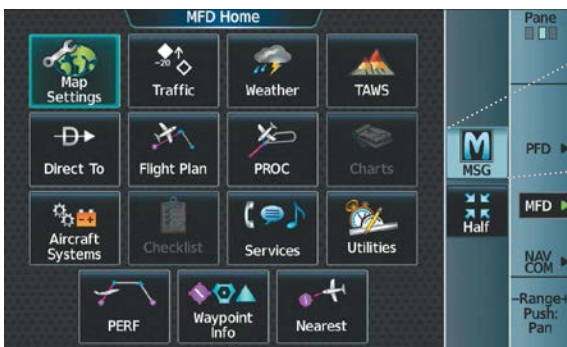
Figure A-7 System Messages Annunciation (Touchscreen Controller)
