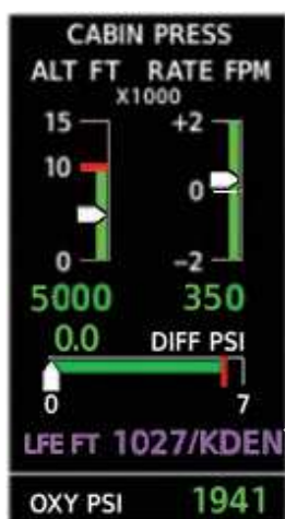
Figure 3-10 FMS LFE on the Cabin Pressure Display
