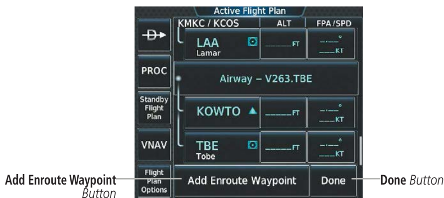
Figure 5-74 Active Flight Plan Screen - Adding a Waypoint to the end of the Enroute segment of the Flight Plan
