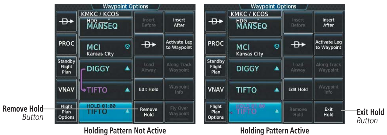
Figure 5-104 Removing a User Defined Holding Pattern at an Active Flight Plan Waypoint
