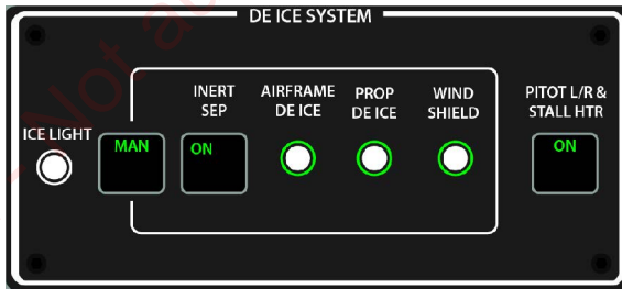
Figure 7.14.3 - DE ICE SYSTEM panel - MAN mode activated
