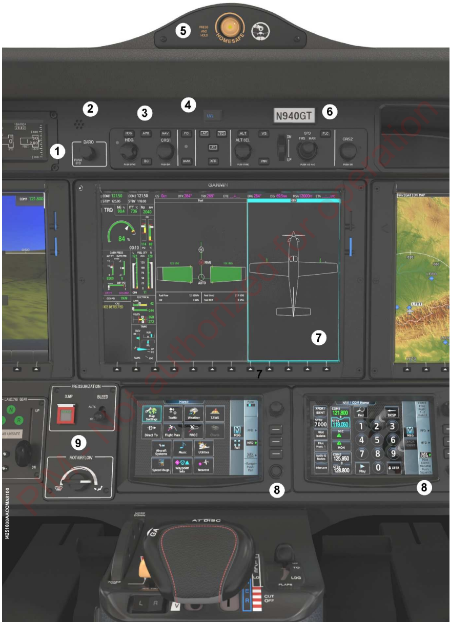
Figure 7.3.4 (2/2) - Central instrument panel (Typical arrangement)
